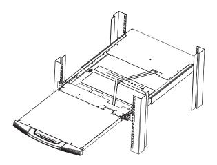
3. Rotate the top panel all the way back to expose the LCD screen.
